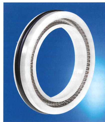
Fig. 1. A spring-supported seal for a ball segment used in an engine cooling water circuit. It is made from modified PTFE, processed by injection molding, and demonstrates the usefulness of this material – for medicinal areas as well (© ElringKlinger Kunststofftechnik)
