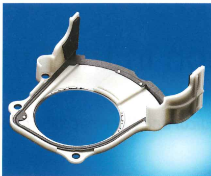
Fig. 2. This component is installed in housing covers in a vehicle engine compartment. It consists of a front cover made from 30% glass-fiber-reinforced polyamide with an encapsulated sealing lip made from a PTFE compound. It also contains a metal insert and is designed for rapid installation (© ElringKlinger Kunststofftechnik)
