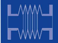
**Pointed, Non-cut Folds** for maximum expansion and low pressures up to 3 bar.
